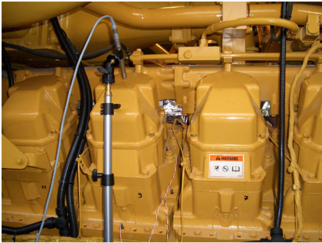
Fig. 4. Vibration and acoustic signal acquisition on the cylinder No. 9 of the CAT G3516B engine.
