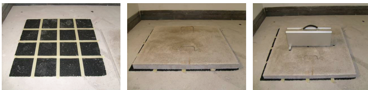
Figure 7. From left to right: picture of the tested acoustic underlay; picture of the concrete slab on the sample; picture of the tapping machine.
