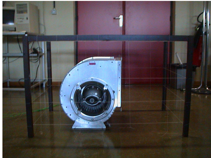
Figure 1: Used Centrifugal Fan with grid for Experimental Study
